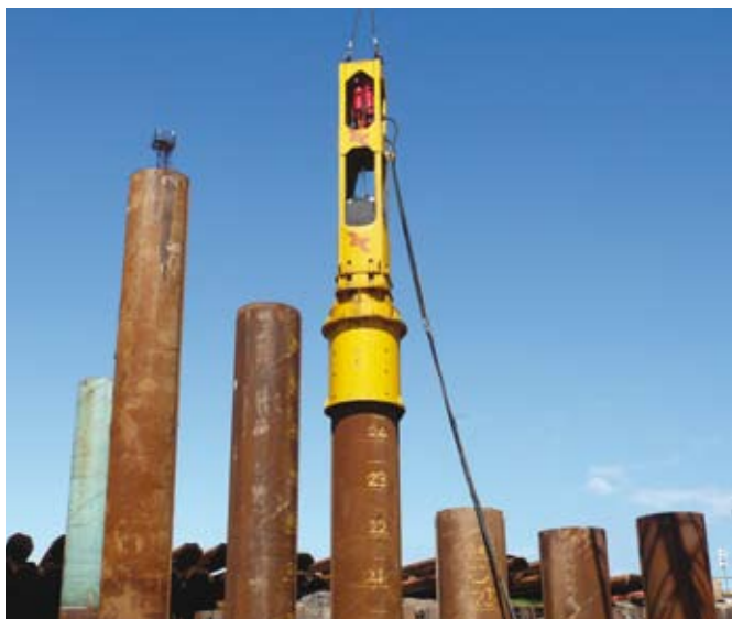
BSP CG210 Hydraulic Piling Hammer. Able Seaton Port, Hartlepool, UK
