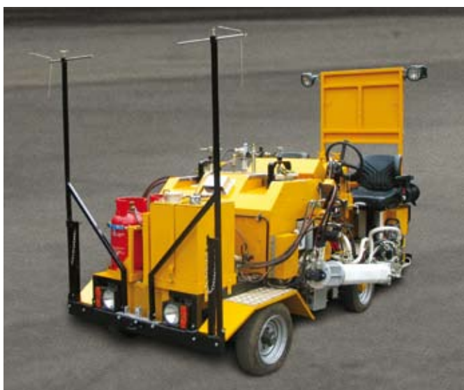
Springwood Engineering – S1100 (Self Propelled) Spray/Extrusion/Rib Thermoplastic Road Marking Machine – versatile for the laying of lines within cities, towns and urban road systems
