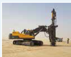
4. BSP Dynamic compactor operating in Dammam, Saudi Arabia.
